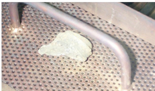
Fig. 2. Stainless steel/tantalum/stainless steel crucible and alloyed metal.
